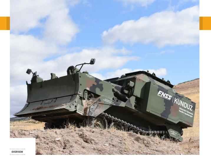
The AACE is an amphibious, armoured, tracked, combat earthmover, designed for the preparation of river banks during river crossing missions. It is capable of performing bulldozing, rough grading, excavating, hauling, and scraping operations.
